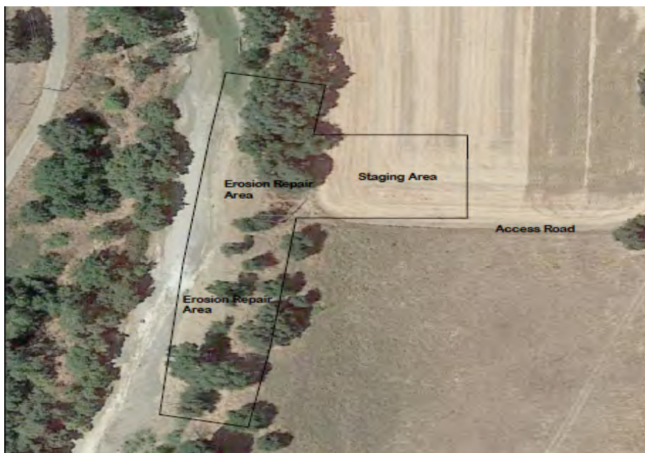
Figure 4. Aerial view of the Freeman Road erosion repair site (~RM 15.75).
